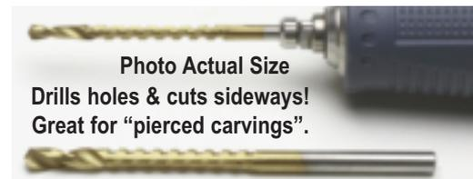
**2-PC MINI SAW DRILL SET** Perfect for "pierced carvings"; these amazing bits drill holes & side cut to shape openings in material up to 3/4" thick. The bits are precision made from special super hard Titanium nitride (TiN) coated HSS steel for heat resistance & long life. Set includes 1 ea. of 3/32" & 1/8" shank (fit standard power tool collets). Lengths: 2" & 2.25".
