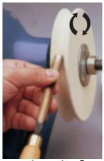
inside edges gouges has always been one of the biggest obstacles to sharpening carving tools. The woodcarvers felt wheel is specially shaped to reach into all the contours of even the deepest gouges & Vtools, to remove burrs & polish to a
