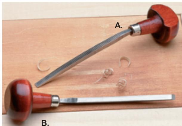
**MULTI-LINE TEXTURE TOOL** Create multi-line texture for hair, fur & feathers with each stroke! Simply push along surface of wood and you'll instantly have 4 or 6 lines of texture. We recommend 6 line tool for carvings smaller than 6", 4 line for carvings larger than 6". Length 5.25". Width 3/16". U.S.A.
