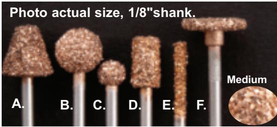
**CARBIDE NUGGET™ BURRS** Shape wood quickly, without the clogging & deep scratches left by other bonded carbide burrs! These burrs are made of virtually indestructible carbide on 1/8-inch steel shanks. There are 6 favorite carving shapes that won't wear out, load up, break down, or overheat. Use to shape all woods, plastic, fiberglass & ceramics (Not for use on metal). Medium grit. Maximum speed 30,000 rpm. Shanks: 1/8", Length: 1.5". USA
