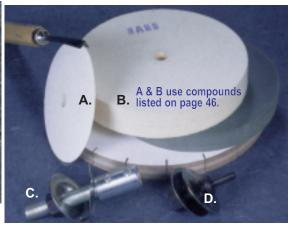
A-B. FELT WHEELS Use for final polishing, deburring, honing to razor sharp edge. Simply charge wheel while running with compound. Made with natural hard 100% wool felt so compound stays on longer. Unlike soft muslin & cotton wheels, hard felt won't round edges & lasts for years. V-edge wheel used for deburring, honing & polishing of V tools & narrow gouges. Mounting arbors below adapt wheels to motors & drills. 3,450 RPM max. Holes: 5/8" with 1/2" sleeve.
