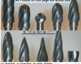
10-PIECE CARBIDE BURR SETS High quality carbide burrs at a great price! Genuine carbide burrs are preferred for carving because they outlast standard steel & "high speed steel" burrs. Teeth are mid depth set for quick stock removal & smooth finish. Use with flex-shafts, micro & other grinders. Maximum speed 30,000 rpm.
