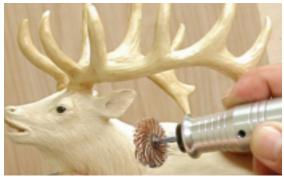
RADIAL BRISTLE DISCS. A radically new approach to sanding by 3M! Aluminum oxide & 3M Cubitron™ are embedded in the plastic bristles. Amazingly, the flexible bristles make wood smooth & remove "fuzzies" left by power carving & burning, without harming the underlying detail! Hole: 1/16"; Diameter: 3/4". Mandrels must be ordered separately.
