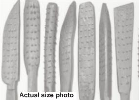
RIFFLER RASPS Riffler rasps are perfect for quickly carving & shaping difficult to reach areas. Ours feature sharp, hand set teeth, forged from properly hardened tool steel (Rc 55). Tough enough to carve stone! Our sets cover most all carving needs. Jumbo & large sizes in coarse grit are best for rapid shaping. All leave light scratches that may be easily removed by fine rifflers. Sets includes favorite carving shapes on double-ended rifflers. Length: 8".
