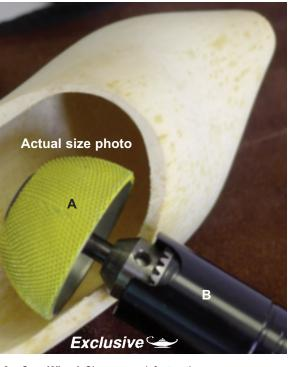
**A. Cup Wheel** Shape wood faster than you ever dreamed possible! To use, simply attach to your favorite 1/4" capacity flex-shaft handpiece or die grinder. The deep radius is great for shaping wood spoons & bowls. Specifications: 1/4" Shank, 1.75" Diameter x 1" width , Max. speed 25,000 rpm. U.S.A.
