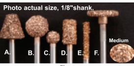
CARBIDE NUGGET<sup>™</sup> BURRS Shape wood quickly, without the clogging & deep scratches left by other bonded carbide burrs! These burrs are made of virtually indestructible carbide on 1/8-inch steel shanks. There are 6 favorite carving shapes that won't wear out, load up, break down, or overheat. Use to shape all woods, plastic, fiberglass & ceramics (Not for use on metal). Medium grit. Maximum speed 30,000 rpm. Shanks: 1/8", Length: 1.5". USA
