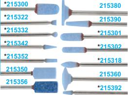
**CERAMCUT BLUE STONES** Fast cutting, perfect for detailing & texturing. We recommend Blue Stones for a smoother finish after using diamond or other cutting burrs. They work better because the abrasive material is ceramic grain, a super tough, fast cutting, non-fused ceramic aluminum Excellent for all woods, also great for hard metal, glass & plastic. Most are fine grit 120 (except 215356 is Coarse 60 grit). 45,000 RPM max..3/32"shanks.Length:1.75". U.S.A.
