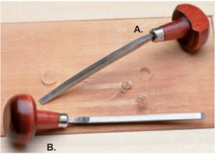
**MULTI-LINE TEXTURE TOOL** Create multi-line texture for hair, fur & feathers with each stroke! Simply push along surface of wood and you'll instantly have 4 or 6 lines of texture. We recommend 6 line tool for carvings smaller than 6", 4 line for carvings larger than 6". Length 5.25". Width 3/16". U.S.A.
