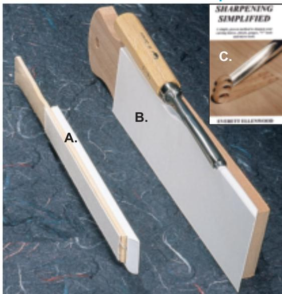
**A. & B. HONE-STROPS** Sharpening your tools to a mirror finish & razor sharpness is easy with the Hone-Strop. Charge strop with strop compound, then rejuvenate a dulling edge on gouge, chisel, knife or achieve that final polish. Revolutionary hard rubberized composition resists wear & will not round cutting edges. Sides specially shaped to sharpen & polish inside V-tools & gouges. Includes instructions.
