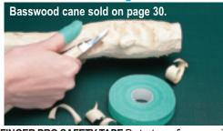
FINGER PRO SAFETY TAPE Protect your fingers against minor cuts, burns & abrasions, without sacrificing comfort! Just wrap around fingers to be protected, sticks only to itself. Super comfortable, it "breathes" & allows free movement. Protects your fingers & improves grip. Essential for small hand held carvings. 3/4"x90' roll.
