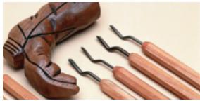
"DOCKYARD" MICRO DETAIL DOG-LEG SET Same high standards as our other micro detail carving sets, Rc 58 blade hardness & razor sharp edges. Dogleg chisels are great for carving hard to reach areas (particularly backgrounds in relief), model making & wherever precise, smooth, cutting is needed. Set includes the 4 most useful Dog-Leg chisels: 2mm, 2.4mm, 2.75mm & 3.25mm. length 5". U.S.A.
