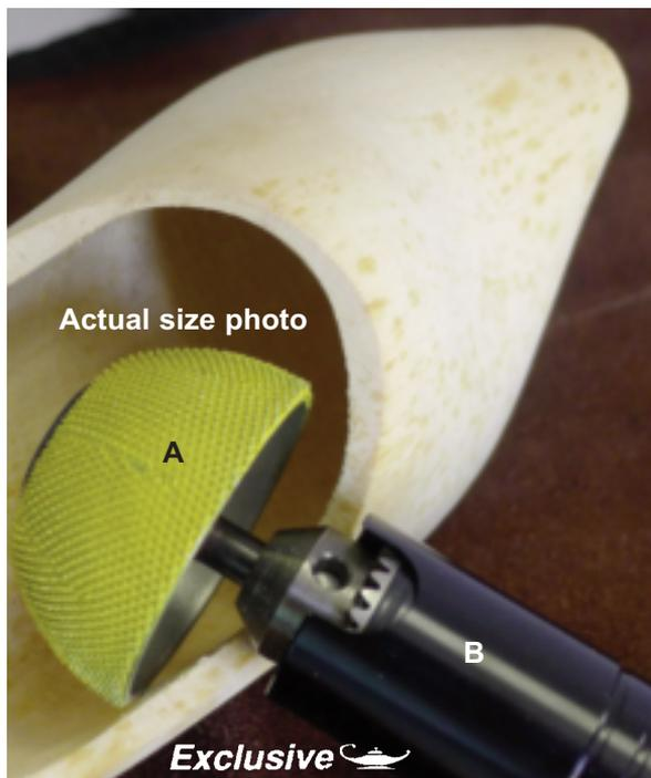
**A. Cup Wheel** Shape wood faster than you ever dreamed possible! To use, simply attach to your favorite 1/4" capacity flex-shaft handpiece or die grinder. The deep radius is great for shaping wood spoons & bowls. Specifications: 1/4" Shank, 1.75" Diameter x 1" width, Max. speed 25,000 rpm. U.S.A.
