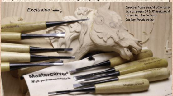
**10-TOOL BASIC SET.** Focused on basic mallet or hand pushed tools for shallow relief, small sculpture & detailing larger carvings. Sets typically include: #1-12mm chisel, #41-6mm 60° V-Tool & the following gouges: #3-6mm, #3-12mm, #5-6mm, #5-12mm, #7-12mm, #9-3mm, #10-6mm, #10-10mm & tool roll. Pre-sharpened. Boxwood handles, Rc 58-62; Length: 9". **401004 10-Tool Basic Set & Roll** \$99.95
