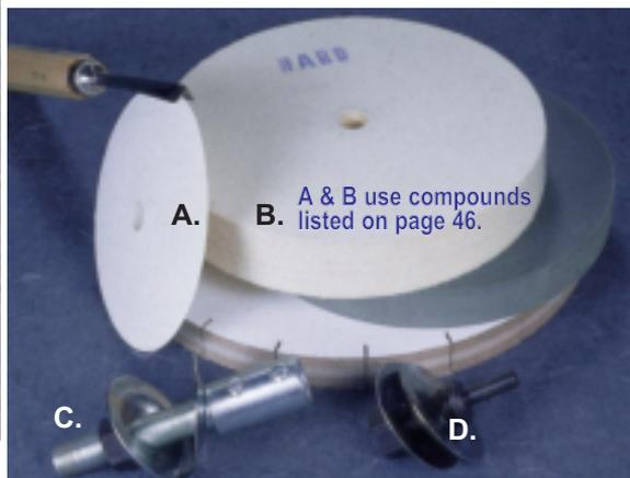
**A-B. FELT WHEELS** Use for final polishing, deburring, honing to razor sharp edge. Simply charge wheel while running with compound. Made with natural hard 100% wool felt so compound stays on longer. Unlike soft muslin & cotton wheels, hard felt won't round edges & lasts for years. V-edge wheel used for deburring, honing & polishing of V tools & narrow gouges. Mounting arbors below adapt wheels to motors & drills. 3,450 RPM max. Holes: 5/8" with 1/2" sleeve.
